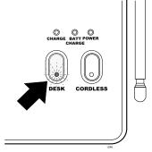
**Note** If the cordless AC Adapter is unplugged or if the Strata CTX system is turned off, the mode automatically changes to the CORDLESS mode.
